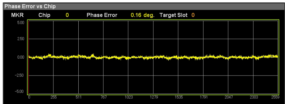
Figure 3.6.4.4-1 Phase Error vs Chip display
